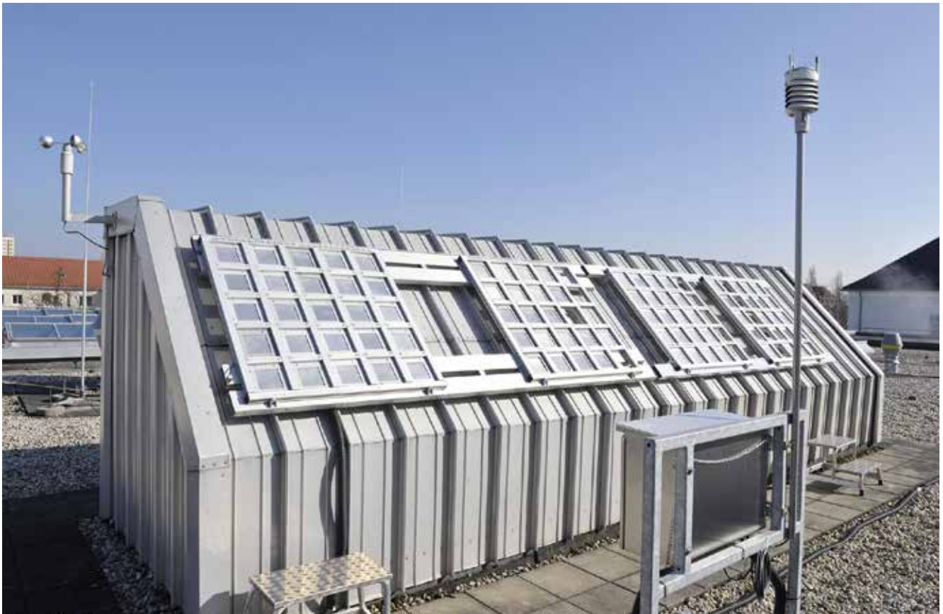
Outdoor weathering test rig on the roof of the Technical Center at the Fraunhofer FEP in Dresden (figures: Fraunhofer FEP)
